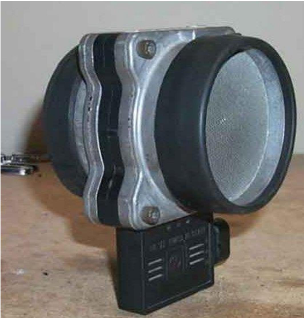
**Figure 4 - Mass Air Flow Sensor. GM LT1 Shown.**
