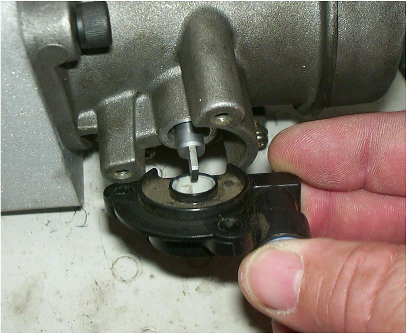
**Figure 2 - Throttle Position Sensor (typical GM)**
