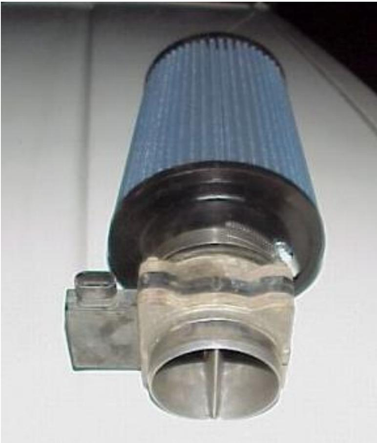
**Figure 5 - MAF sensor with air filter fitted.**
